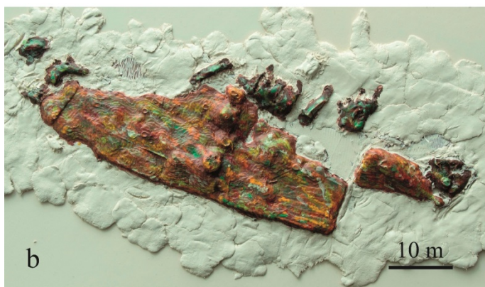
Figure 1. (a) A multibeam image of the site SS Vilhelm Krag; (b) A 3D image, after digital processing and editing.
